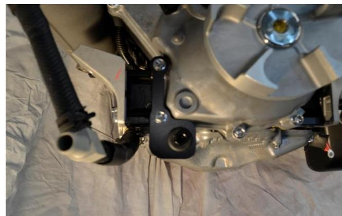
Remove the 14mm head exhaust pipe mounting bolt.
