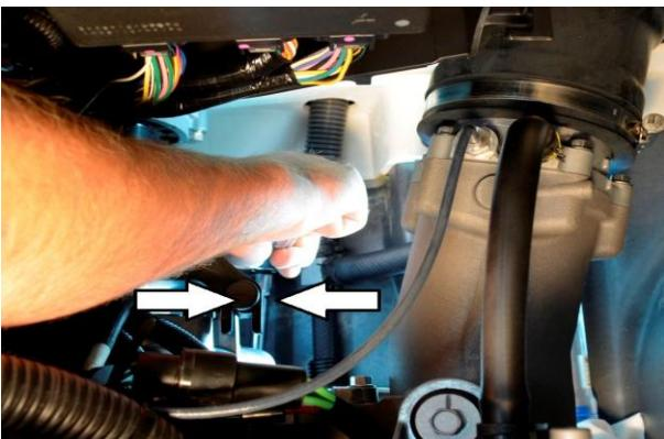
Slide the supplied crush washer over the threaded end of the black hex adaptor & install in the oil pan where the drain plug was. **Tip:** Place a very small amount of grease between the hex adaptor & the crush washer. This will hold the crush washer in place while installing the black hex adaptor.
